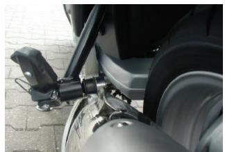
**Production** The muffler is secured to the mounting location through the use of a **Solution**: large washer together with a longer screw.
